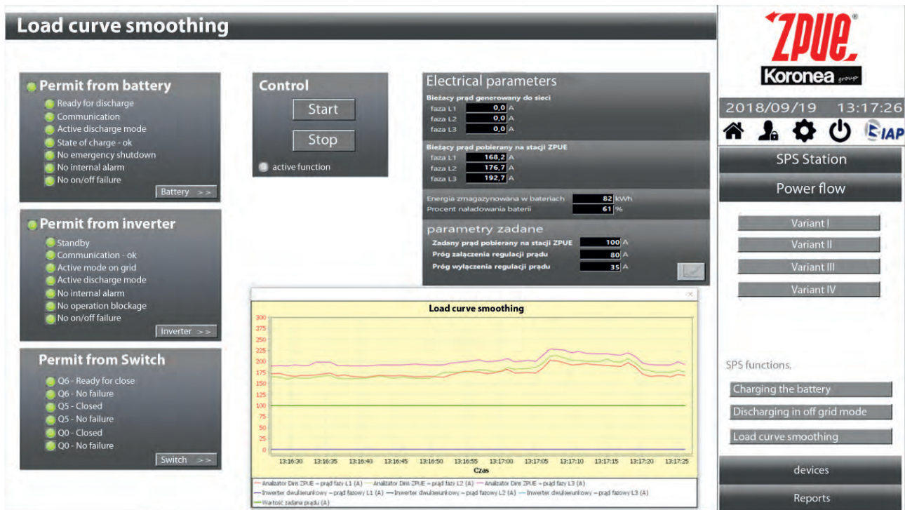
Example SCADA system screen for active function monitoring
